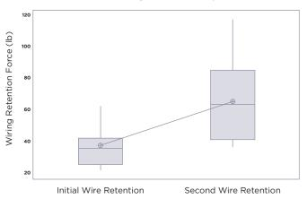
Upon installation, a 10 AWG THHN stranded wire required 40 lb of force to disengage. After exposure to vibration per the UL standard, 65 lb of force was required to disengage.
