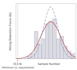
Compared to the UL minimum requirement for wire retention, EdgeConnect screwless termination offers superior strength.
